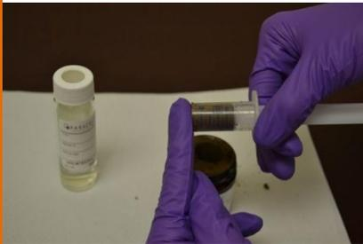
Depress the plunger to the 12 mL mark to **lightly** compress the soil into a 5 mL (2.5 cm) core. A 5 mL core represents approximately 5 g dry weight.
