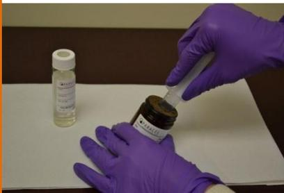
Sampling directly from the split spoon (or soil auger), draw the plunger past the 12 mL mark, push the barrel of the syringe into freshly exposed soil and compact the soil to fill the barrel. It may take more than one attempt to fill the barrel completely.
