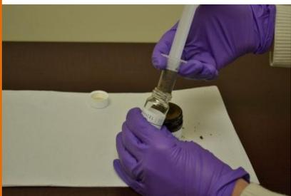
Remove the cap from the methanol vial, wipe any soil or debris from the outside of the syringe and align the barrel with the vial opening. Care should be taken not to insert the syringe directly into the vial.
