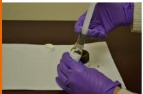
Remove the cap from the methanol vial, wipe any soil or debris from the outside of the syringe and align the barrel with the vial opening. Care should be taken <u>not</u> to insert the syringe directly into the vial.
